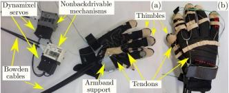
Two sets of fingers were chosen to be actuated: (1) index finger and middle finger and (2) thumb, since with this configuration is possible to perform most types of graspings commonly used to execute daily tasks.
